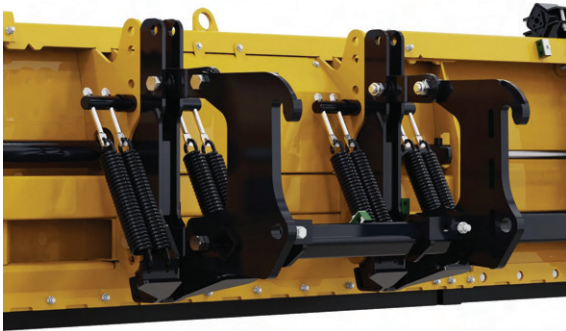
Constant Pressure System & Mechanical Float
